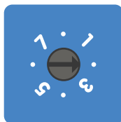
Rotary switch set to position 2
