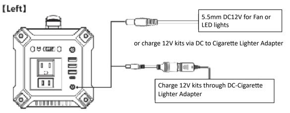
\*Note: The 5.5mm DC output and the car port output voltage ranges between 9V~12.6V. DC output voltage drops while battery capacity drops due to chemical characteristics of the battery. If your appliance is not built-in input voltage stabilizing function, it may shutdown when input voltage is too low. If your 12V devices cannot work due to high input voltage, please read the device manual or consult the device manufacturer to get the input voltage range of your device.
