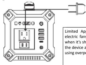
Limited Appliance Wattage <300W for lamps, electric fans, TV's, and more! AC will shutdown when it's short circuited or is overloaded. Unplug the device and the unit will recover automatically using overpower protection in just a few seconds.
